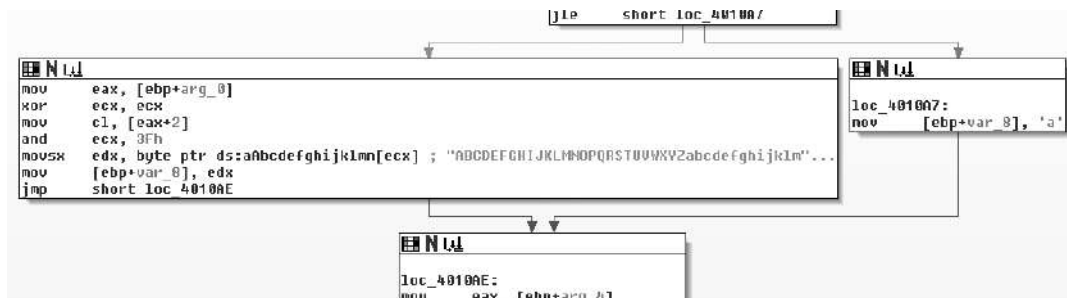
Figure 14-2L: Base64 encoding function (0x401000) with alternative padding
